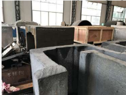
PF clamps rough forgings
