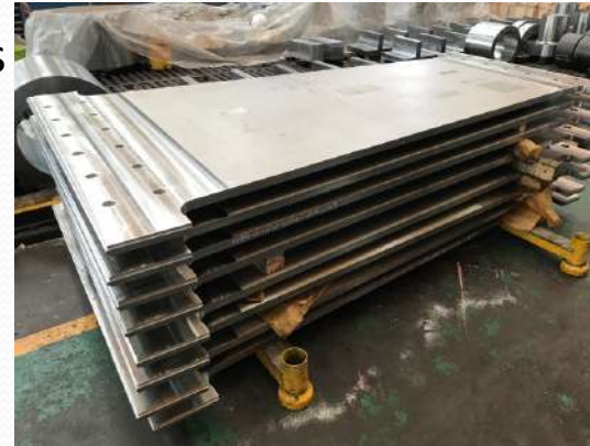
PF clamps rough forgings
