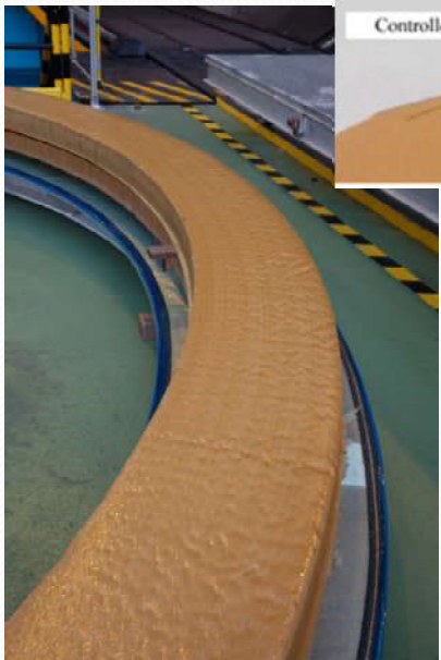
Full diameter prototype ring after curing, showing wrinkles
