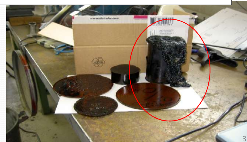
Lab-scale thermal runaway of cyanate ester
