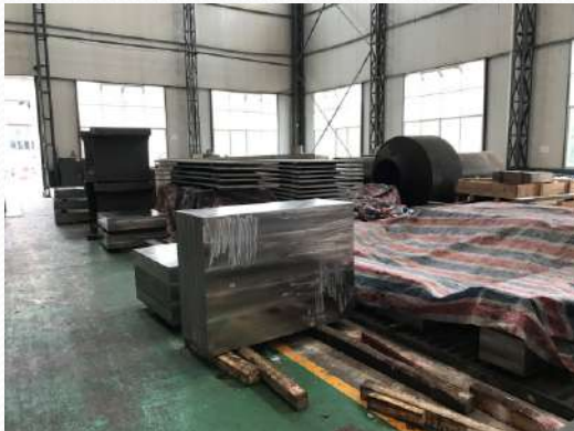
Behind: PF clamps (left), TF GS plates (right), PF6 plates and blanket shielding blocks (front)
