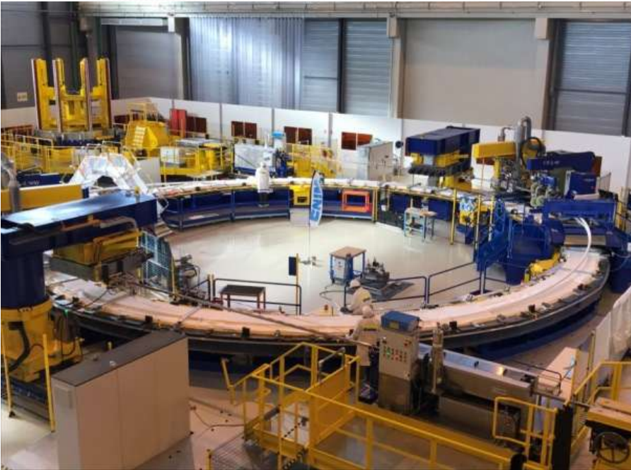
PF5: 2 nd DP(DP8) Winding Completed
